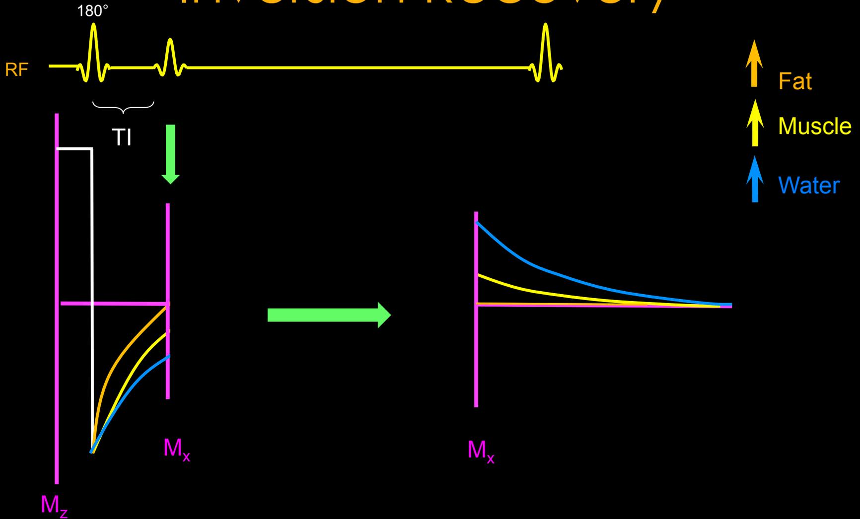
TI chosen to null undesired signal (~150ms for fat @ 1.5T)
